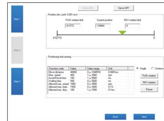
Easy auto-tuning using position JOG and self-adjustment
