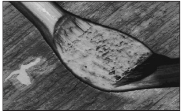
Figure 1. Ultrasonic Wire Bonded Joint. 0.001” aluminum wire bonded to ½ ounce electrodeposited copper on RT/duroid 6010 material. No attempt to clean the copper foil surface was made, but the result is still a good joint.
